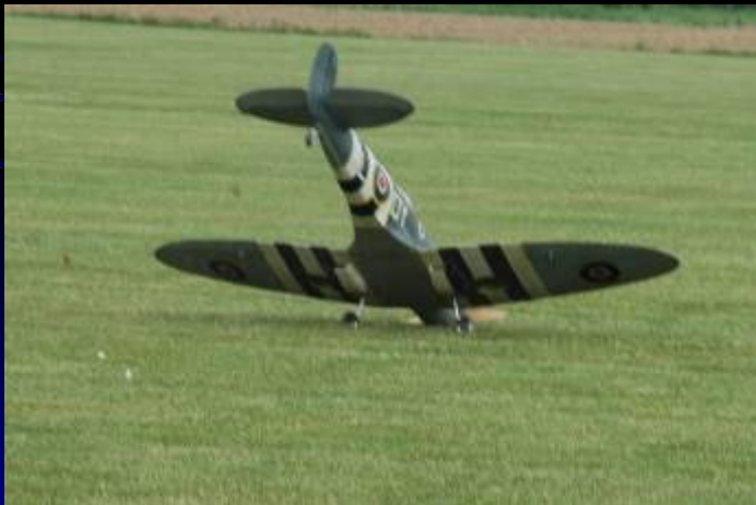
Elliptical for uniform lift across wing
